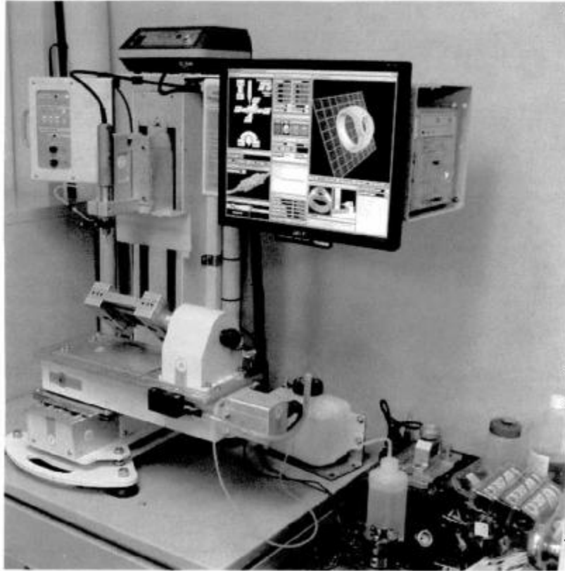
↑ Revvo 540b Milling System – wax models for casting ↓
